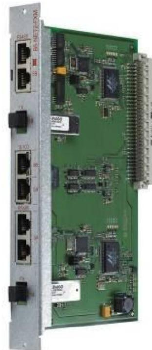
Fig. 8 B5-NET2-FXM network board
