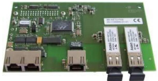
Fig. 22 B6-NET2-FXS network unit
