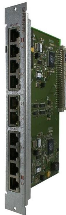
Fig. 2 B5-NET4-485 network board
