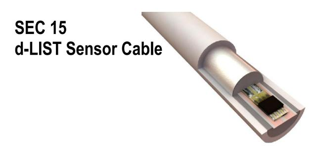
The hermetically sealed sensor cable contains temperature sensors which, depending on the application, are placed at selectable intervals. The sensors are electrically connected by a flat flexible cable.
